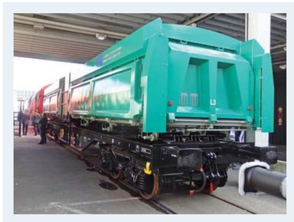
CROATIA: A self-propelled wagon fitted with a 55 kW diesel generator and hydraulic transmission giving it the ability to move around worksites at up to 100 km/h under remote control has been developed by RZV Čakovec and partners.
